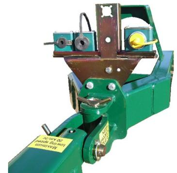
*TR Air Seeder Hitched with Optional Rigid A-Frame Pull*
