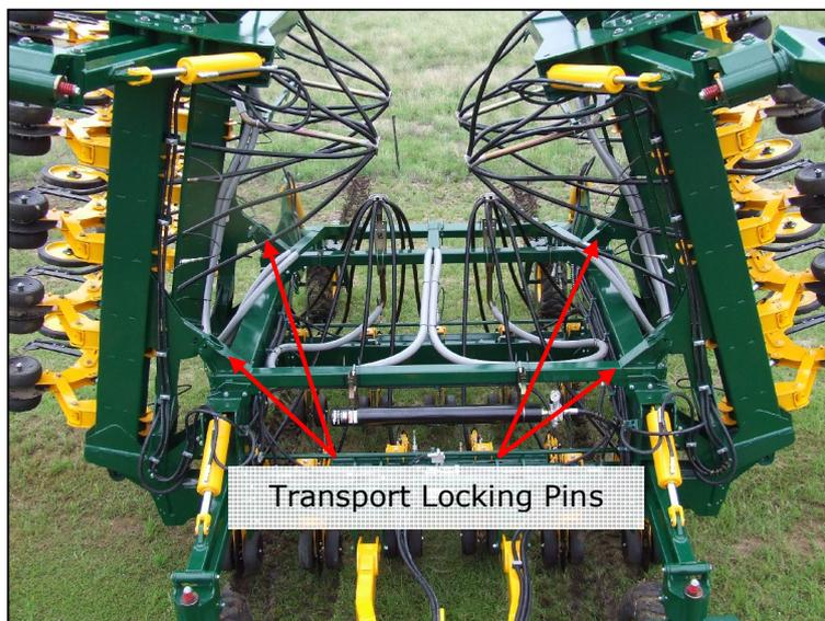
When folding for transport ensure that wings are fully folded and **wing locking pins securely in place.**
